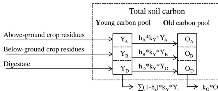
Figure 1. Introductory Soil Carbon Balance Model (ICBM)
